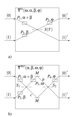
FIG. 1: A universal quantum interference device operating on a qubit can be realized by a 4-port interferometer with two input ports  $|0\rangle$ ,  $|1\rangle$  and two output ports  $|0\rangle'$ ,  $|1\rangle'$ ; a) realization by a single beam splitter S(T) with variable transmission T and three phase shifters  $P_1, P_2, P_3$ ; b) realization by two 50:50 beam splitters  $S_1$  and  $S_2$  and four phase shifters  $P_1, P_2, P_3, P_4$ .
