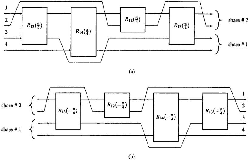
FIG. 1. Experimental realization of (a) the encoding stage of a two-component two-share configuration by an array of effectively two-dimensional beam splitters depicted as boxes. The decoding stage (b) is just the encoding stage (a) in reverse order, with inverse beam splitters.
