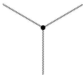
Figure 3.1: Schematic illustration of a star polymer, consisting of a core particle and three attached linear polymer arms.
