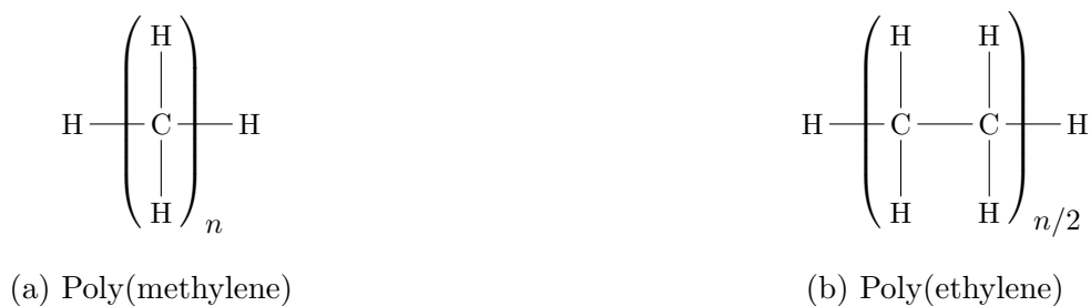
Figure 2.1: Two equivalent representations of a polyethylene macromolecule with n C-atoms and 2n H-atoms (plus two more for the end monomers), with equivalent degrees of polymerization n and n/2 , respectively; in (a), the monomer unit is \text{CH}_2 , while in (b), it is \text{C}_2\text{H}_4 . The latter representation is more traditional, as is the source-based name polyethylene , compared to the structure-based name poly(methylene) . 14
