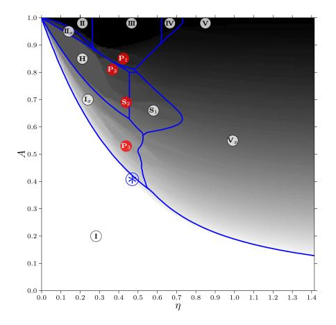
FIG. 6. The same as in Fig. 5, now in terms of the order parameter  $x = n_2/n$ . The following gray-scale encoding was used: x = 0 corresponds to white, and x = 1/2 to black. Note that the value x = 1/3 is of particular relevance (see regions surrounding the labels of structures H, S<sub>2</sub>, and S<sub>1</sub>).
