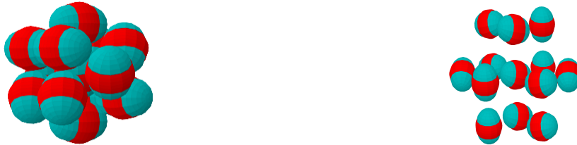
Figure 54: The unit cell of the investigated fcc-structure formed by spatial and orientational ordered IPCs is shown at a typical particle density (left) and at extremely large distances so that the orientation of the particles can be seen (right).
