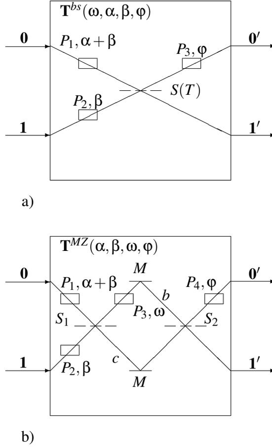
**Figure A1.** A universal quantum interference device operating on a qubit can be realized by a 4-port interferometer with two input ports  $\mathbf{0}, \mathbf{1}$  and two output ports  $\mathbf{0}', \mathbf{1}'$ ; a) realization by a single beam splitter  $S(T)$  with variable transmission  $T$  and three phase shifters  $P_1, P_2, P_3$ ; b) realization by two 50:50 beam splitters  $S_1$  and  $S_2$  and four phase shifters  $P_1, P_2, P_3, P_4$ .
